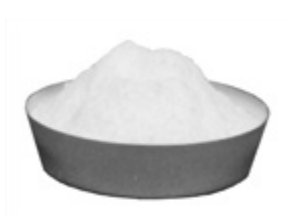
Low Density Powders Tend to Overflow
