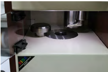
Integrated Die of Choice Expedites Pellet Formation And Eliminates Die Handling
