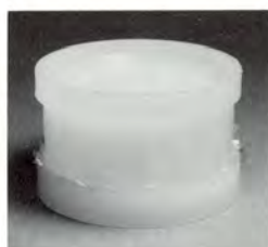
Figure 11 Diagram of push-plunger XRF sample cup.
