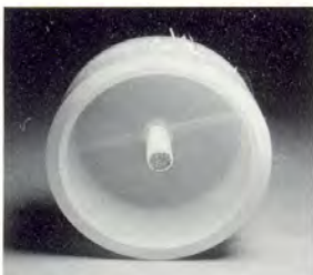
Figure 6 Diagram of 1400 Series cup with microsample mounting feature.
