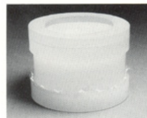
Figure 10 Diagram of convertible closed-open cell cups.
