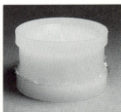
Figure 11 Diagram of push-plunger XRF sample cup.
